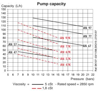
Data shown take into account a wear margin. Do not oversize the pump when selecting the gear capacity.
